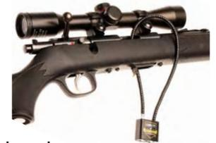
Remove the bolt from the rifle. Insert the cable through the ejection port and out through the end of the receiver assembly. To lock: With key turned to farthest clockwise position, insert loose end of cable into padlock. Turn key counterclockwise and remove key. Check that cable is secure.
